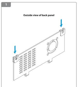
Align the vibration damping pads with the screw holes in the back panel and wrap them around the panel, making sure not to cover the screw holes.
