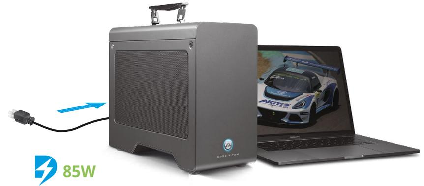
This device supports power delivery (PD), providing up to 85W of power to laptops that support charging from a 15 to 85W power source (e.g. **Late 2016 MacBook Pro**). This allows you to recharge the battery even when the laptop is not connected to its power adapter.
