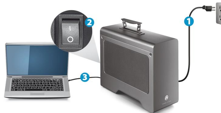
Turn on the computer, plug in the power cord (1), turn on the power (2) and then connect the Thunderbolt cable to the computer (3) to turn on the device. Note: The fan for the power supply is temperature controlled and turns on only when needed.
