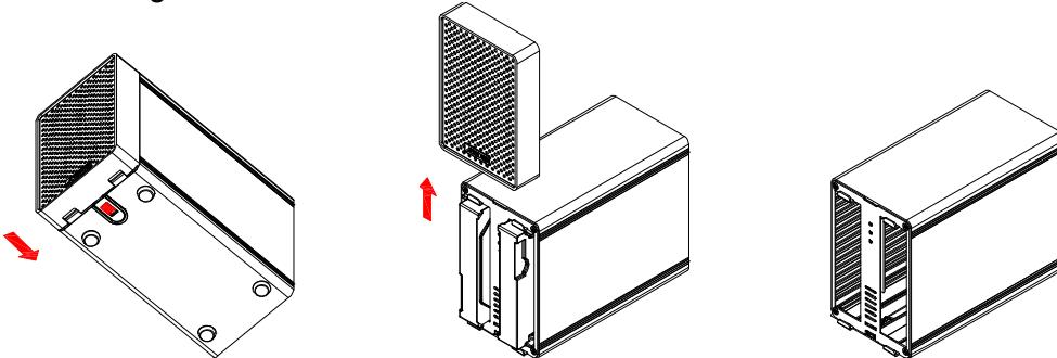
2. Install the hard drives as illustrated below with the top of the drives, where the label is located, facing each other. Push the drives lightly into place and then replace the front panel.
